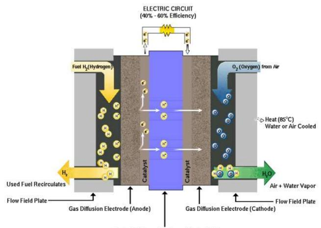
Proton Exchange Membrane (Electrolyte)
